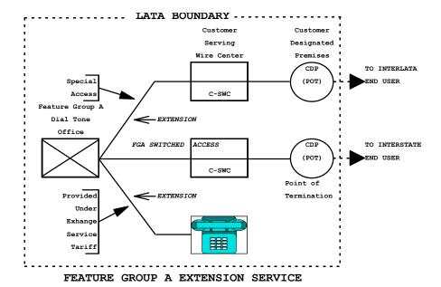
In the above example, two CDPs are utilized to better illustrate the concept. From a practical standpoint, both the Switched Access and Special Access Services could be routed via the same CDP.
