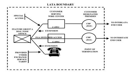
In the above example, two CDPs are utilized to better illustrate the concept. From a practical standpoint, both the Switched Access and Special Access Services could be routed via the same CDP.
