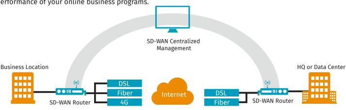
**Hybrid:** A hybrid WAN solution augments an existing MPLS network with SD-WAN using affordable broadband connections. This allows you to customize connectivity by location and need and gives you a cost-effective way to easily add more bandwidth without sacrificing security. This type of solution also enables your business to keep up with rapidly increasing bandwidth demands without having to rip and replace your existing WAN infrastructure.
